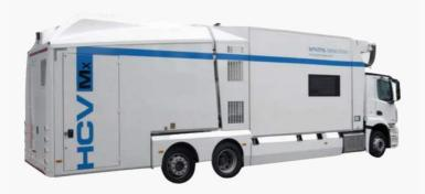
The **HCVM** X-ray screening system is designed for ease of operation and can be driven from location to location and be ready for use in less than 30 minutes.
