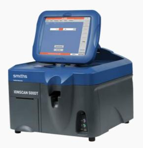
The IONSCAN 500DT is a highly sensitive desktop trace detector used to accurately detect and identify a wide range of military, commercial and homemade explosive threats and common illegal/controlled narcotics.
