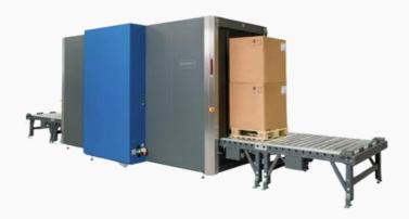
The HI-SCAN 145180-2is pro is a state-of-the-art X-ray inspection system for scanning objects up to 145 cm x 180 cm (57"/71") [W × H]. Due to the compact footprint and large tunnel dimensions, the imaging system is perfectly suited for the inspection of air cargo, freight and palletized goods.
